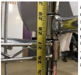
Basin height is important for comfortable use and in order to meet ADA accessibility specifications. With wheels installed the middle shelf should be 27" above the ground and handle installed directly above that. This results in a basin top height of 34". The top and bottom shelf should be installed all the way up and down respectively.
