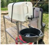
A rubber strap secures the water jug and "jack chain" is used to hang the back of the basin to pitch the water toward the drain.
