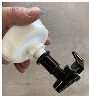
The high flow spring loaded toggle (HFSLT) valve used for the spigot has 3/4" UNF threads (straight) and the tote cap has 3/4" FPT (tapered). A 3/4" FPT to 1/2" FPT to 3/4" MPT adapter works well to connect them with a layer of Teflon tape on the 3/4" MPT side of the adapter and 2 layers on the 3/4" UNF threads of the spigot. Also note that the tote cap has a 3/4" knockout that needs to be drilled for water to flow. We used a 3/16" hole to restrict water flow.
