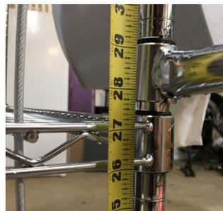
Basin height is important for comfortable use and in order to meet ADA accessibility specifications. With wheels installed the middle shelf should be 27" above the ground and handle installed directly above that. This results in a basin top height of 34". The top and bottom shelf should be installed all the way up and down respectively.
