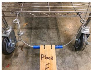
The foot pedal is assembled by creating a loop in the cable. The left side is attached to the frame and the right side is threaded up to the spigot. The cable runs between the wires on the middle shelf or through screw eyes / bolts.
