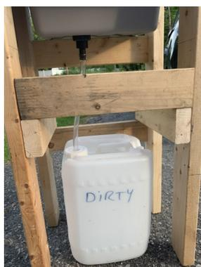
The flush mount basin drain has a hose barb fitting that makes it easy to connect to a collection tote with a vinyl hose. The hose is passed through the tote cap where the 3/4" knockout has been removed. Label the totes "clean" and "dirty" to help ensure they are only used for one purpose.
